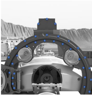
Figure 5. Detected bolts in the Bit Carousel
